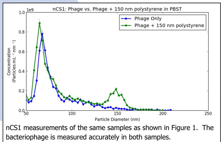
In summary, the nCS1's unique implementation of microfluidics-based resistive pulse sensing demonstrates consistent and high resolution measurements of particle size and concentration *independent* of the particle material. All materials can thus be measured equally well.
