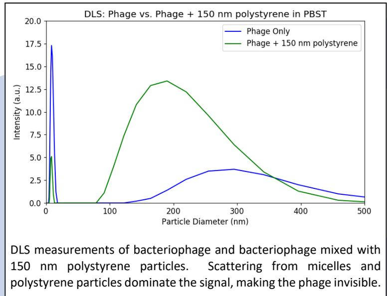
DLS measurements of each sample are shown in Figure 1. In each case, a peak in the scattering intensity is seen near 8 nm diameter resulting from the polysorbate micelles in solution. The 150 nm diameter polystyrene beads in sample 2 are detected by DLS, with measured diameter near 190 nm. **DLS fails to detect the phage in either sample.**
