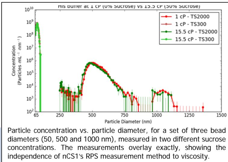
Particle concentration vs. particle diameter, for a set of three bead diameters (50, 500 and 1000 nm), measured in two different sucrose concentrations. The measurements overlay exactly, showing the independence of nCS1's RPS measurement method to viscosity.
