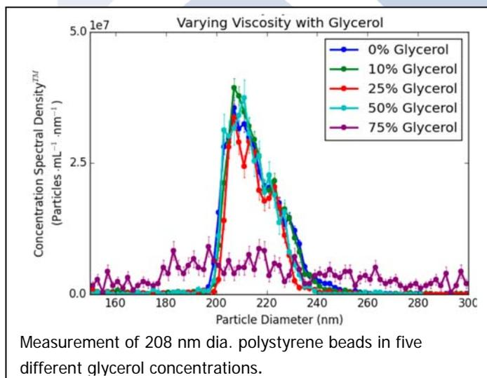
Measurement of 208 nm dia. polystyrene beads in five different glycerol concentrations.
