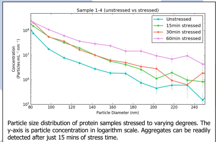
A clear trend of increasing particle concentration with increasing stress time was observed over the full range of measured diameters, although the relative change for small diameters increased significantly more than for large diameters (see below).
